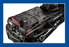
LOCK & RIDE® PLATFORM Integrated design allows for maximum storage, with or without passenger seat. A huge 85lb. (38.5 kg.) carrying capacity and. integrated Lock & Ride mounting system holds cargo box and other storage accessories.
