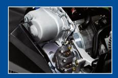
ALPHA TRANSMISSION Provides smooth shifting and drive ranges to suit even the most extreme conditions or situations. 1200 lb. towing capabilities with High, Low, Reverse, and Neutral.
